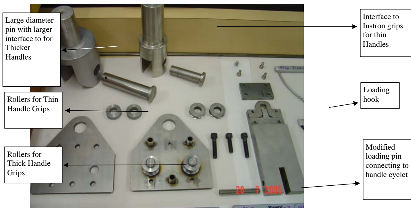
Figure 2. Components of Modified Test Fixture
